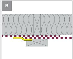
• We recommend (e.g. for flat roofs, wide joists or extremely high insulation material weight) installation of the membrane in the direction of the rafters, sealing in the rafter area and longitudinal installation of the battens.
