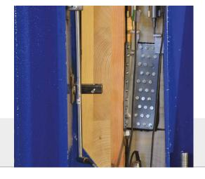
Experimental data on the static performance of a timber-to-steel connection with ALADIN interposed
