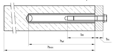
$t_{\text{fix}}$  = thickness of fixture
