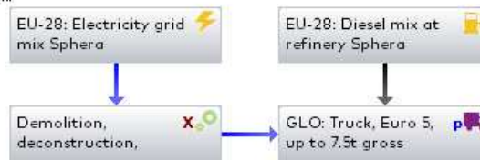
Figure 10: GaBi plan for C1 and C2 modules
