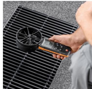
**Digital 16 mm vane anemometer testo 416**
